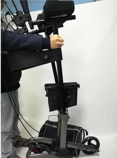
3. Insert the tubes with the arthritis supports into the frame parts of the stand. Loosen the knob screw on the tube support here, push or pull the handle tube to the desired height (holes for fixing) and tighten the knob screw again. Make sure that the same height is set on both sides. The brake cables run parallel to the frame.
