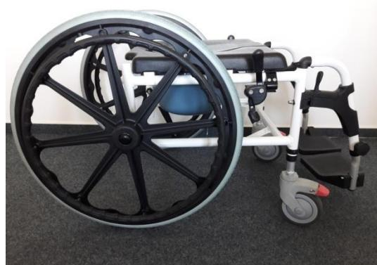
5. Secure the brakes by tilting forward the brake pedals on the rear wheels. On the front wheels, press down the red pedal.
