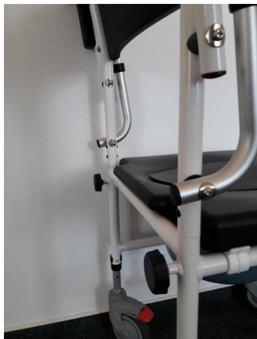
6. Insert the lower tube ends of the backrest in the openings at the back of the frame and secure them using the two knob screws. Fold the armrests down.
