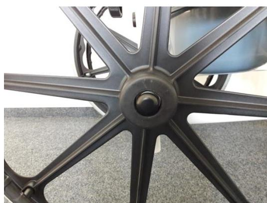
To release the rear wheels, press the quick-release mechanisms in the centres of the wheels.
